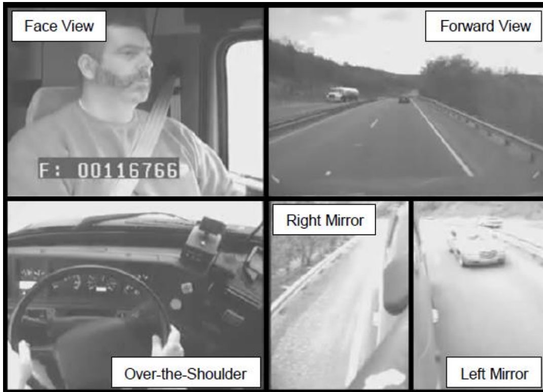
Figure 2. Five NDS camera images multiplexed into a single image
