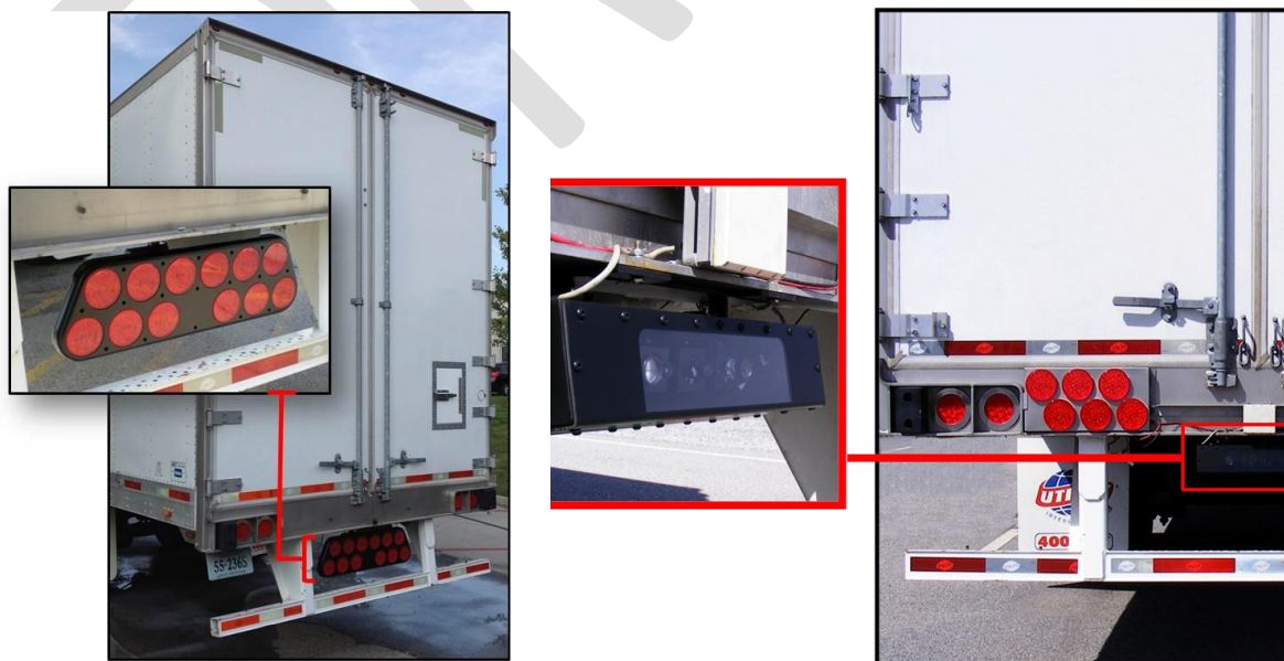
Figure 4. Left, rear-lighting configuration developed and tested in Bowman et al. (2010). Right, radar to detect following vehicle TTC and initiate the flashing alert when a pre-determined threshold has been breached (Schautd et al., 2010).
